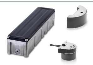
The SeaBat F50 is a high-resolution forward-looking sonar system operating at 200kHz or 400kHz that illuminates a wide 140° horizontal sector ahead of the sonar head assembly. The SeaBat F50 may be mounted on a surface vessel, submarine, AUV or ROV and is available in depth ratings up to 6000 meters.
