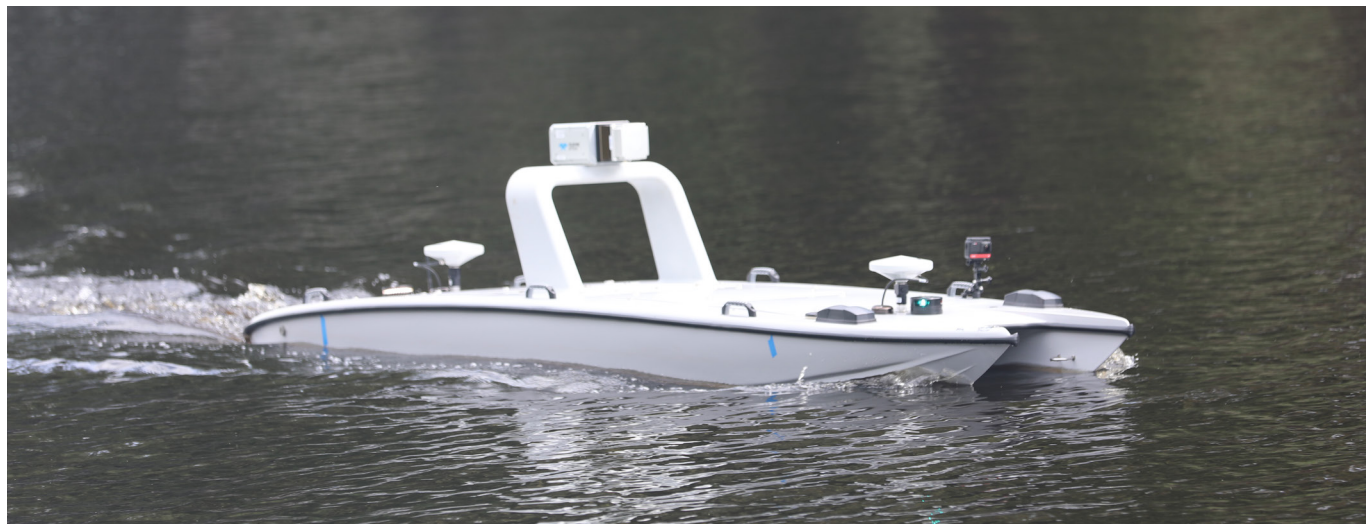
Fully loaded unmanned Mantas T12 vessel with multibeam T20 and laser scanner CL-360 collecting synchronized and accurate 3D data from the Black Creek river
