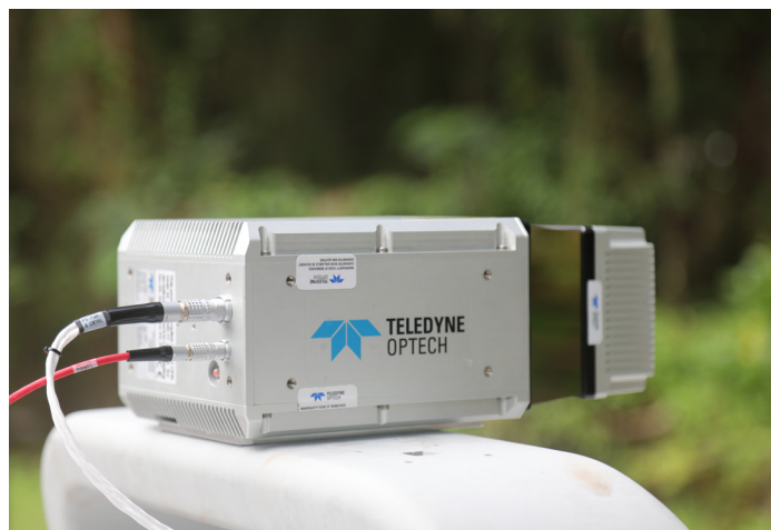
CL-360 laser scanner from Teledyne Optech collecting topographic data from the MARTAC Mantas T12
