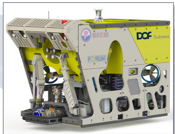
FORUM XLX-C Heavy Duty ROV supplied by Forum Energy Technologies
